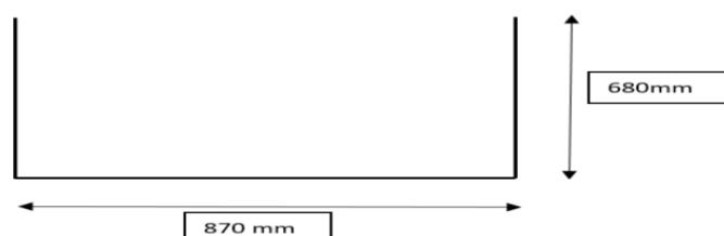
Figure 7: Cross-Section of the Concrete Pipe Trenches
